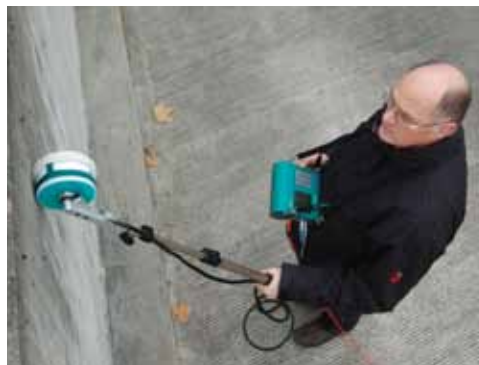
1-Wheel Electrode for fast scanning of large areas
